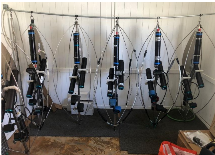
Figure 5 Six units of the Azor drift-cam used during the 2023 deep-sea surveys on board RV Arquipélago and MT Physeter.
